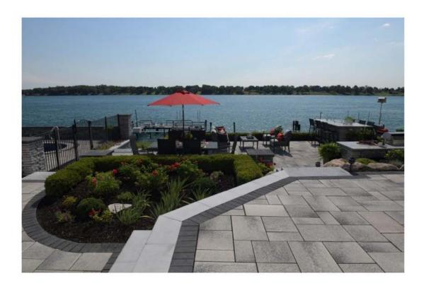
With five compatible sizes, Umbriano pavers can be configured in a variety of laying patterns to create different looks. Pattern sheets in PDF or PAT format are available on the Unilock website. Note that a vacuum placement tool is recommended when placing the large 16" x 16" or 24" x24" stones. The Unilyft paver laying assist machine is ideal for this purpose.
